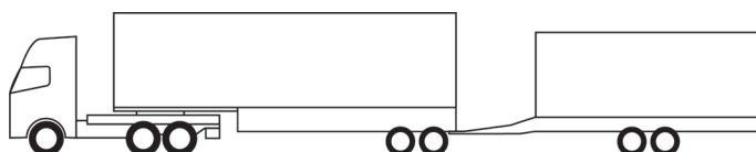
Figure 3 — tractor + A-semi + centre-axle trailer
