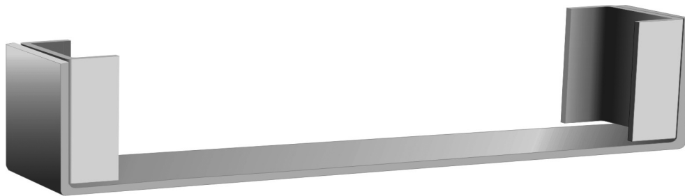
Figure 2 — Specimen jig to hold sandwiches
