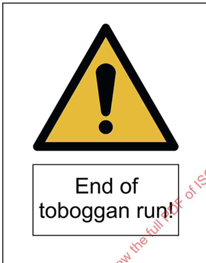
Figure A.4 — General warning sign (ISO 7010-W001) with additional text — Safety statement "End of toboggan run"
