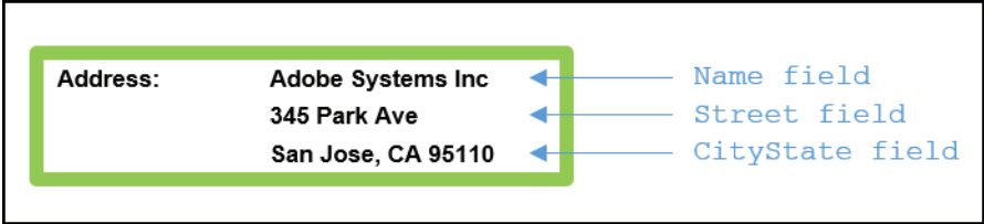
Figure 3 — PDF representing an address label showing example form field names
