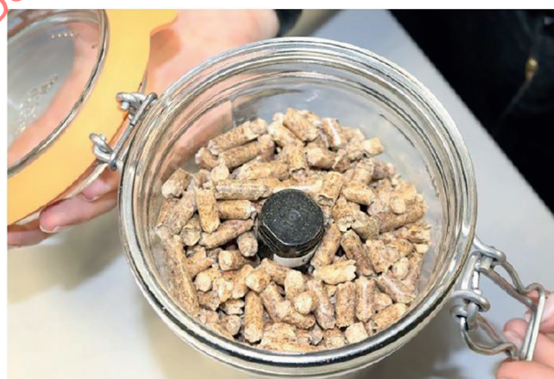
b) Head of the CO data logger sticking out from the pellet bulk after filling the container to the 750 ml mark
