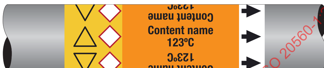
Figure C.5 — Example of a pipe marker with a hazardous content according to an SDS and risk assessment, the warning signs and GHS pictograms on the yellow safety identification colour, the flow direction indicator in black on a white background and, as additional safety information, the temperature of the content of the pipe
