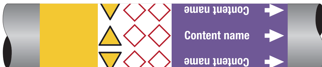
Figure C.12 — Example of a pipe marker with a hazardous content according to an SDS and risk assessment, the warning sign and GHS pictograms on a white background and the flow direction indicator in the contrast colour on the basic identification colour
