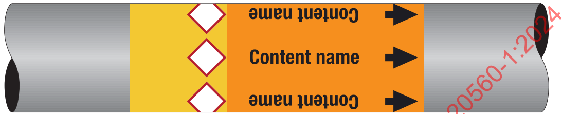
Figure C.10 — Example of a pipe marker with hazardous content according to an SDS, the GHS pictogram on the yellow safety identification colour and the flow direction indicator in the contrast colour on the basic identification colour
