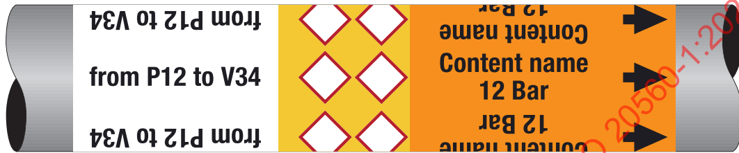
Figure C.6 — Example of a pipe marker with hazardous content according to an SDS, the GHS pictograms on the yellow safety identification colour, the flow direction in the contrast colour on the basic identification colour and, as additional safety information, the pressure of the content of the pipe and from-to information
