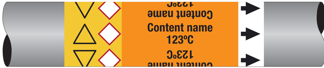
Figure C.5 — Example of a pipe marker with hazardous content according to an SDS and risk assessment, the warning signs and GHS pictograms on the yellow safety identification colour, the flow direction indicator in black on a white background and, as additional safety information, the temperature of the content of the pipe
