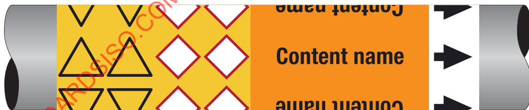
Figure C.3 — Example of a pipe marker with hazardous content according to an SDS and risk assessment, the warning signs and GHS pictograms on the yellow safety identification colour and the flow direction indicator in black on a white background
