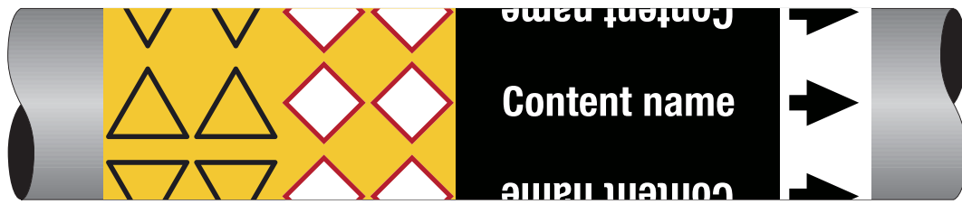
Figure C.9 — Example of a pipe marker with hazardous content according to an SDS and risk assessment, the warning signs and GHS pictograms on the yellow safety identification colour and the flow direction indicator in black on a white background
