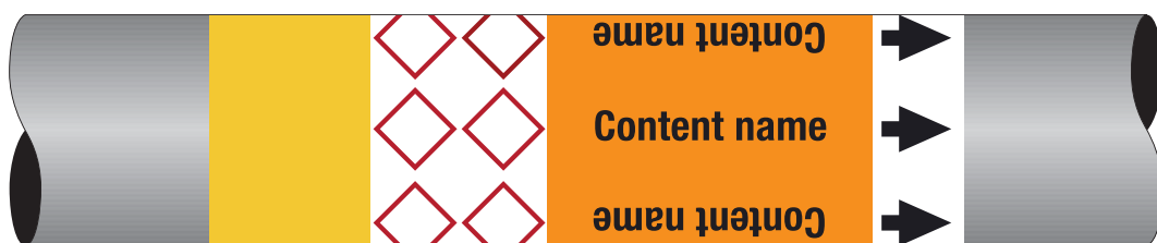
Figure C.4 — Example of a pipe marker with hazardous content according to an SDS, GHS pictograms on a white background and the flow direction indicator in black on a white background
