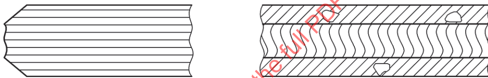
Figure 16 — Arrissed edge (with blank spots)
