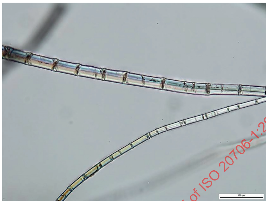
Figure A.2 — Knots — Longitudinal view of ultimate flax (LM)
