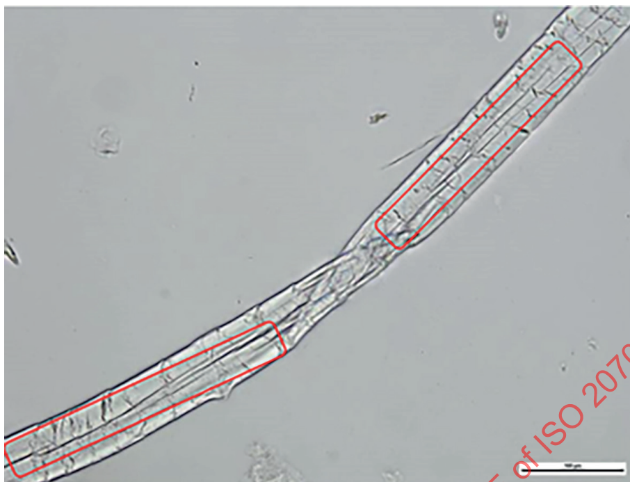
Figure C.2 — Longitudinal striates, fibre twist — Longitudinal view of ramie (LM)
