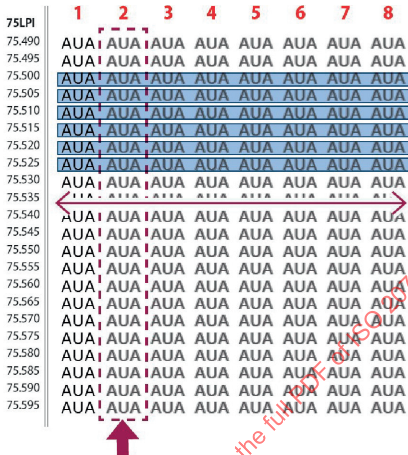
Figure B.6 — Representation of the search for the line where the pattern is clearly observed from the left column to the right column to estimate the pitch of the lenticular lens
