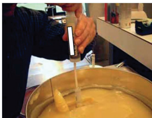
Figure B.5 — Filling the syringe with the help of vacuum, here generated by a larger syringe
