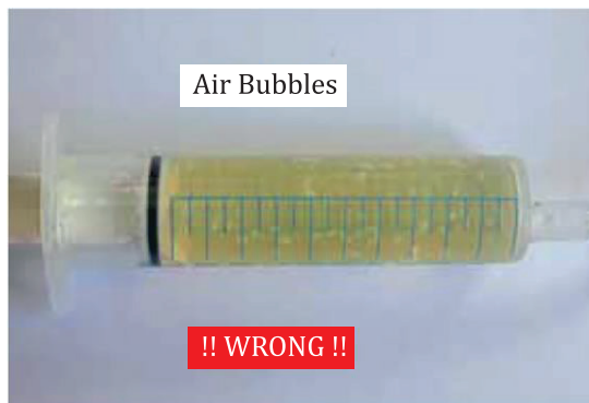
Figure B.3 — Invalid sample with bubbles
