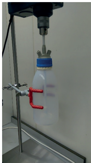
Figure A.2 — Stirring rod blades inside bottle
