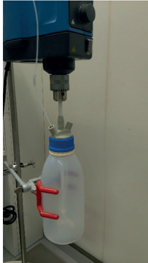
Figure A.3 — Aeration of the suspension
