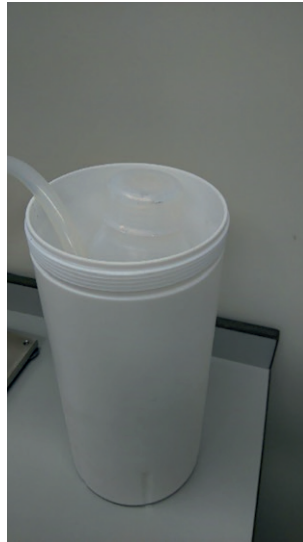
Figure A.5 — Sealed bottle of extraction mixture in container with screw cap
