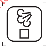
Figure A.1 — Example of graphical symbol for jet stream washing (ISO 7000-3890)
