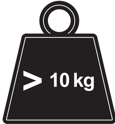
Figure 5 — Example of graphical symbol for parts weighing more than 10 kg (application of ISO 7000-1321B)
