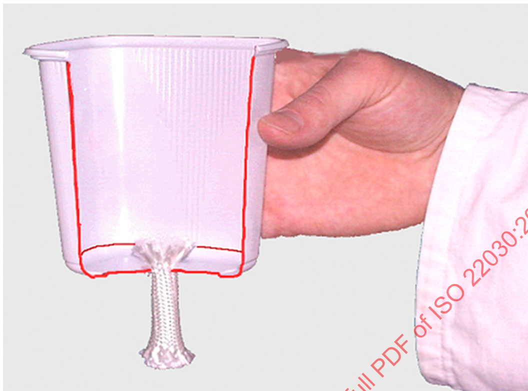
Figure 1 — Example of a test vessel with fibreglass wick
