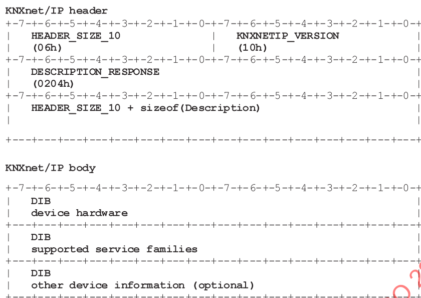
Figure 29 — DESCRIPTION_RESPONSE frame binary format
