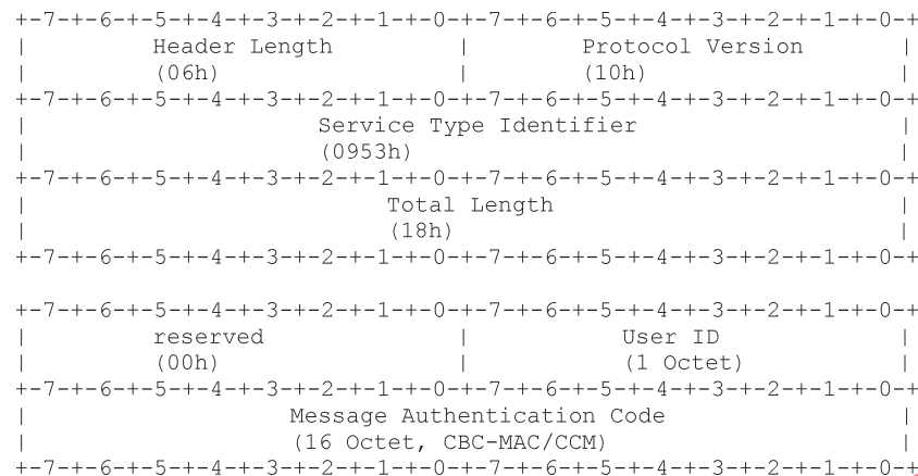
Figure 94 — Binary format of the KNXnet/IP session authenticate frame
