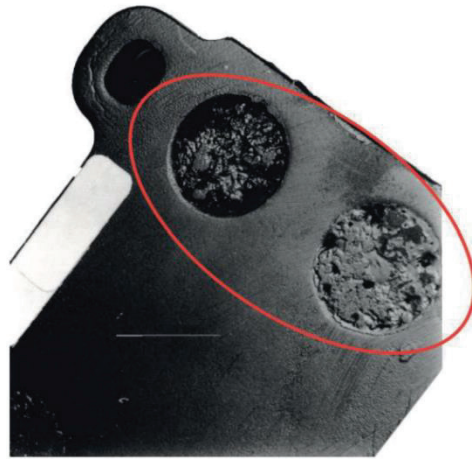
Figure 6 — Poor consolidated spigot holes
