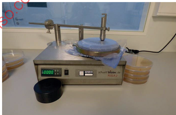
e) Assembly specimen-donor-HDPE, fixed between the two rings placed over the Petri dish on the turntable and the steel finger placed on the test assembly just inside the brim of the petri dish
