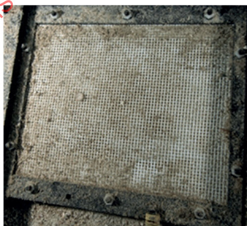
Figure A.1 — Film specimen fixed between two plastic frames and covered with plastic mesh (2 mm × 2 mm)
