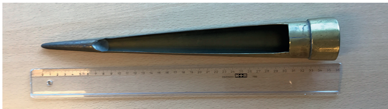
Figure A.3 — Second example of sampling horn for sampling of bags
