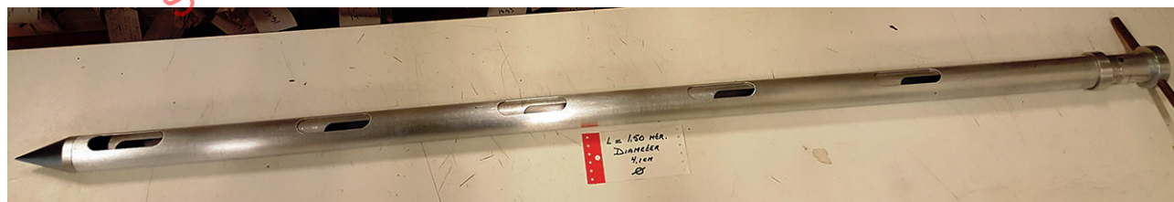
Figure A.4 — Example of a sampling spear for sampling of bulk
