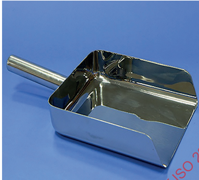
Figure A.5 — First example of a sampling scoop for sampling of bulk
