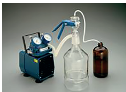
Figure 1 — Example vacuum filter set-up
