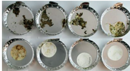
Figure 2 — Example of filter paper decomposition, after oven drying, over incubation period
