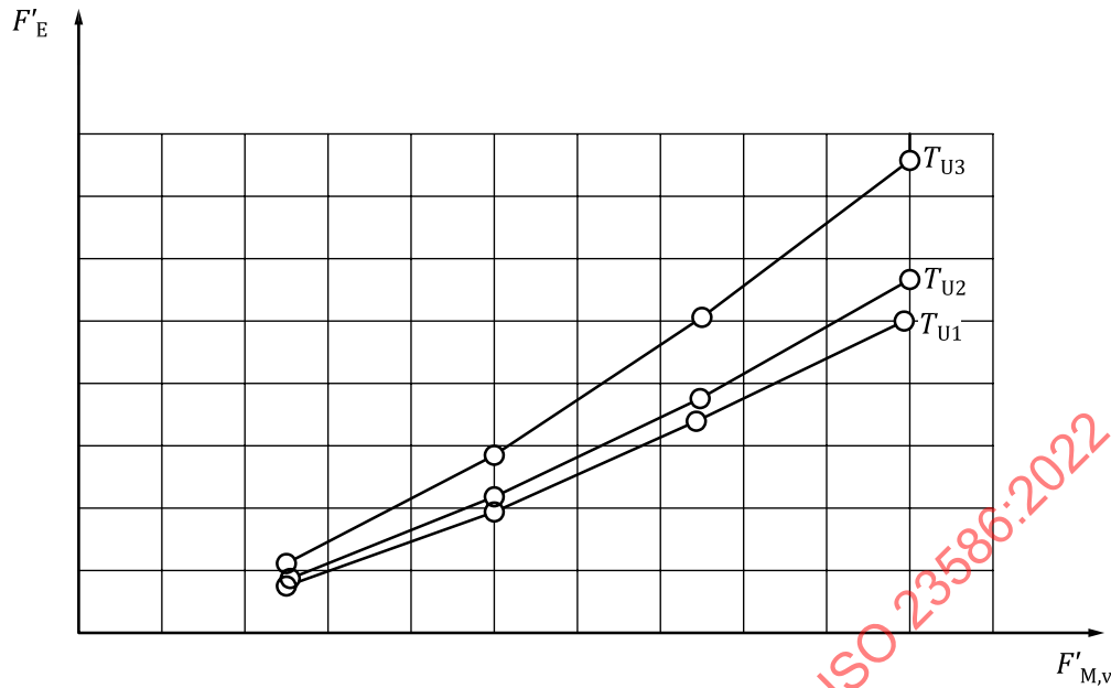
Figure 2 — Example for the variation of the width related indentation rolling resistance F'_E depending on the width-related vertical force F'_{M,v} under consideration of the ambient temperature T_u
