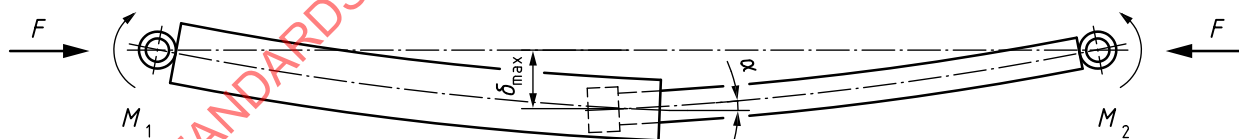
Figure 16 — Cylinder with end moments from axle frictions and angular misalignment
