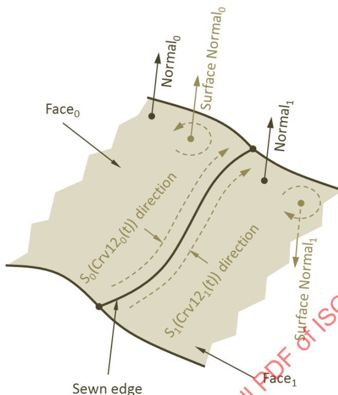
Figure 166 – Sewn Faces (normals of the underlying surfaces are not conformed: Turned 0 (FALSE) ≠ Turned 1 (TRUE))
