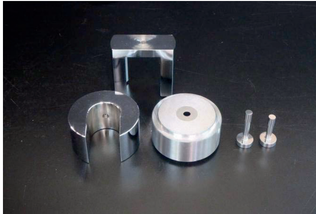
Figure B.2 — Metal mould
