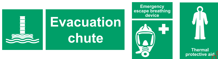
Figure 5 — Examples of combination signs using explanatory text panel supplementary signs (with and without internal borders) (ISO 7010-E055, E029 and E056)
