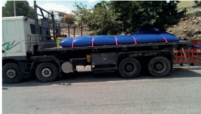
Figure B.7 — Flexible tank strapped on a flat-bed truck
