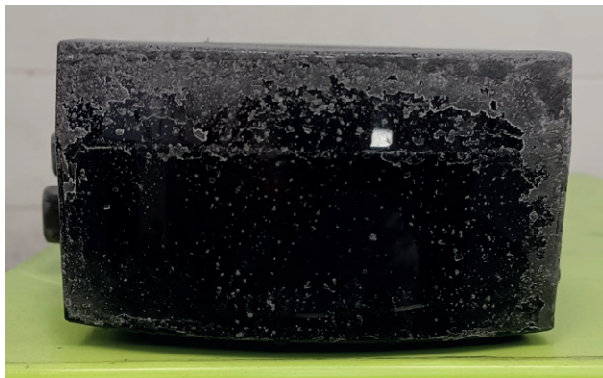
Figure 9 — Example of sensor surface after drying (with remaining contaminant)
