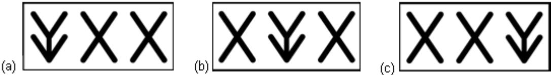
Figure 4 — “Lane Change” signs
