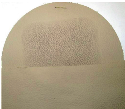
Figure A.1 — Example of soiling test results with the abrasion holder
