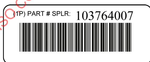
Figure 1 — Bar code symbol example with Data Identifier
