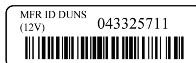
Figure F.1 — Example using DUNS® Number in bar codes
