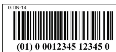
Figure 2 — Bar code symbol example with Application Identifier
