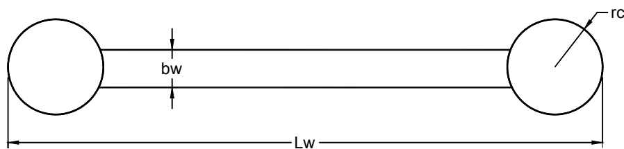
Figure 93 — Circular Columns Embedded in walls
