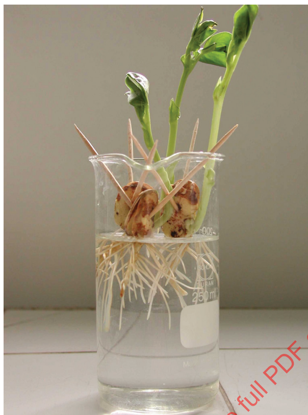
Figure 2 — Method of aqueous exposure of the Vicia faba seeds
