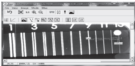
c) Radiograph of a duplex wire IQI on the detector in the free beam area (1 mm Cu filter in front of X-ray tube)
