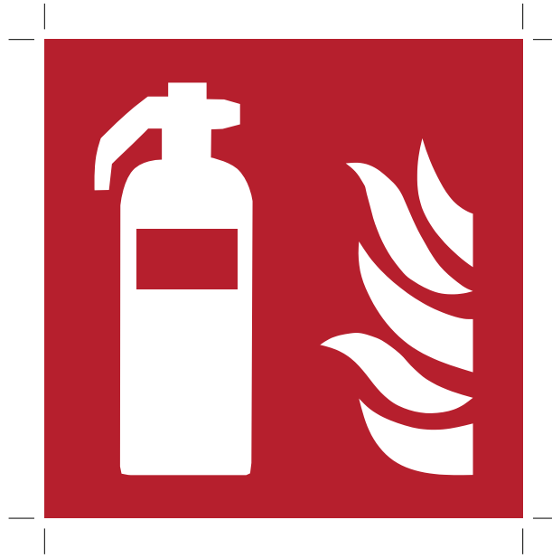
Figure 6 — Fire extinguisher (ISO 7010-F001)
