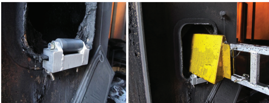
Figure 12 — Roller support clamped to side port of drain - Section of a multi-sloped screen
