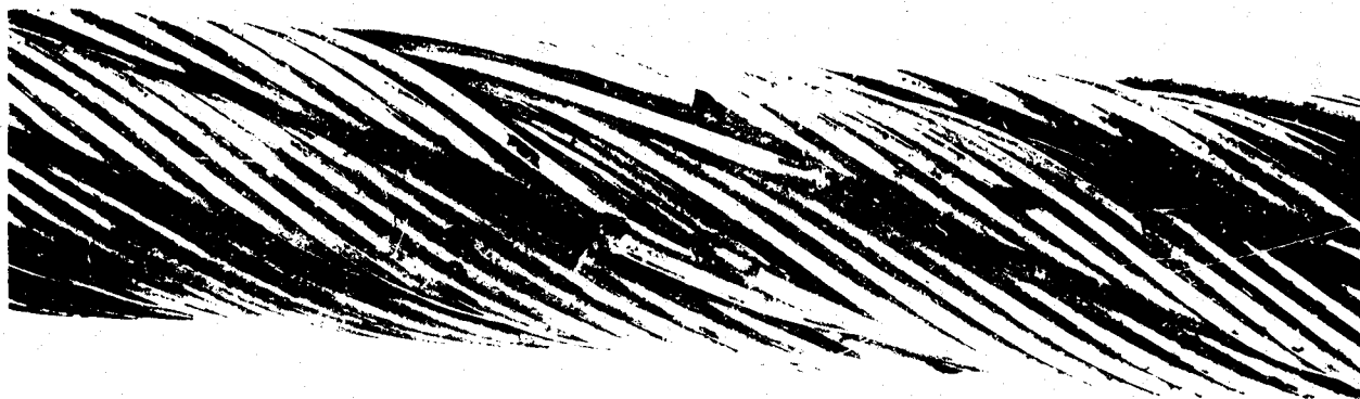
Plate 3 — Wire breaks in one strand, associated with slight wear in a Langs lay rope — justification for further operation if this condition represents the worst condition (fractured wires should be broken out so that the end is at the strand gusset; this prevents further damage to the adjacent wires)
