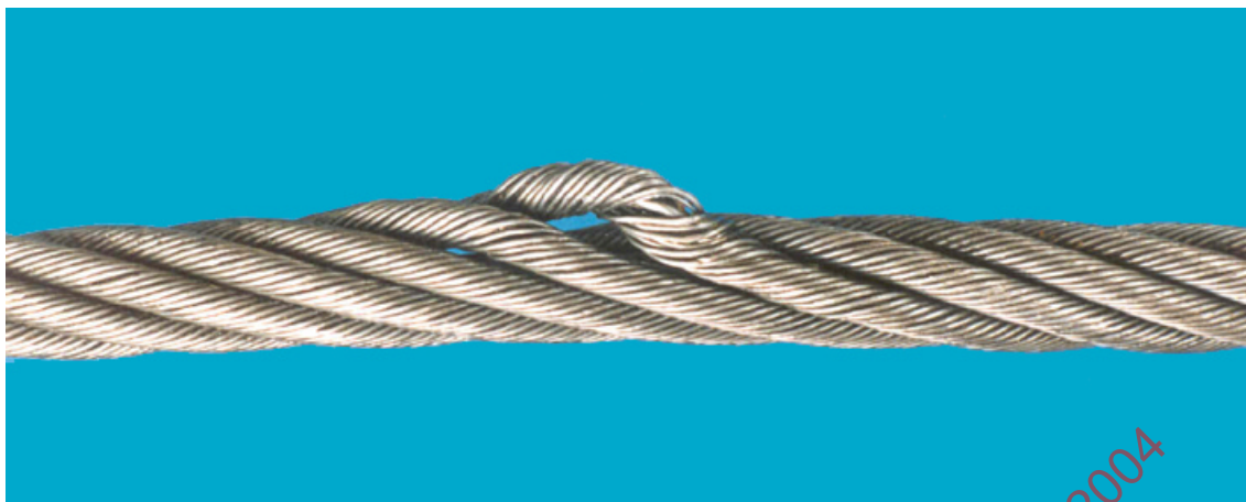
Figure D.4 — Strand protrusion/distortion
