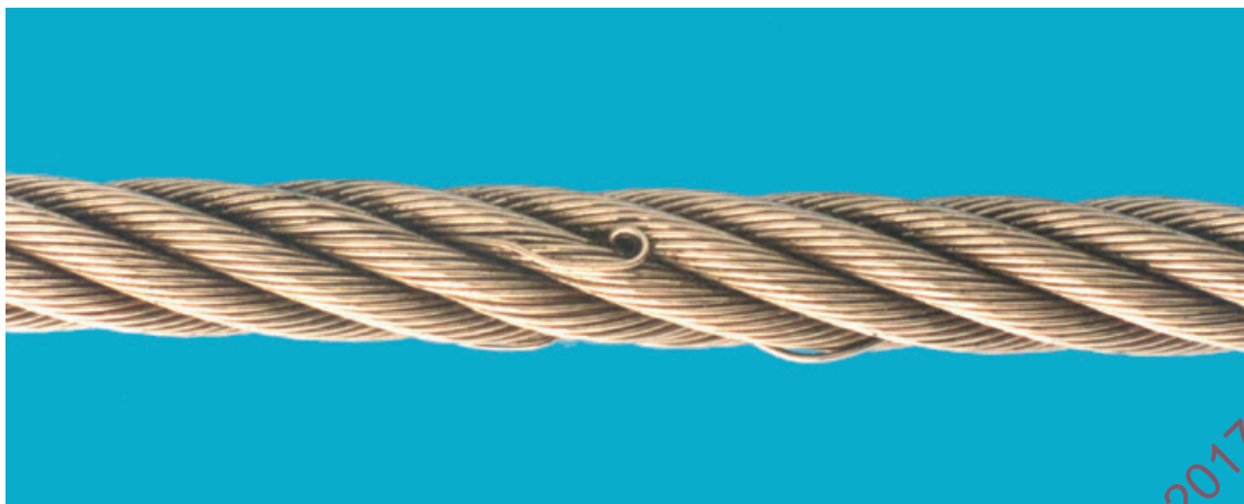
Figure B.14 — Wire protrusion
