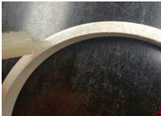
Figure 5 — Example application of Sealant to Bottom of Plastic Ring
