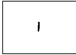
a) Maximum size allowed for a non-relevant indication for severity level LP 5b
