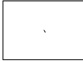
a) Maximum size allowed for a non-relevant indication for severity level LP 1b
