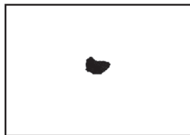
a) Maximum size allowed for a non-relevant indication for severity level SP 5
