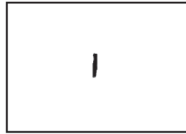
a) Maximum size allowed for a non-relevant indication for severity level LP 4b
