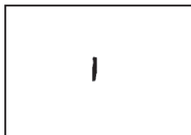
a) Maximum size allowed for a non-relevant indication for severity level LP 4a
