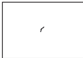
a) Maximum size allowed for a non-relevant indication for severity level LP 3b
