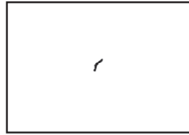
a) Maximum size allowed for a non-relevant indication for severity level LP 3a
