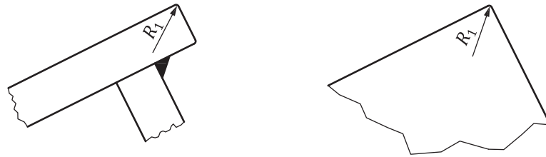
Figure 5 — Radius of curvature, R_1 , at the beta edge shown, as examples, for fabricated and machined cones
