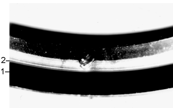
Figure 5 — Inclusion: foreign material
