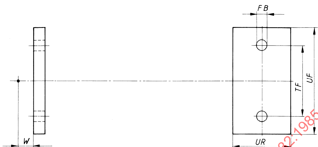
Figure 2 — Head rectangular flange (two hole) mounting (MF8)
