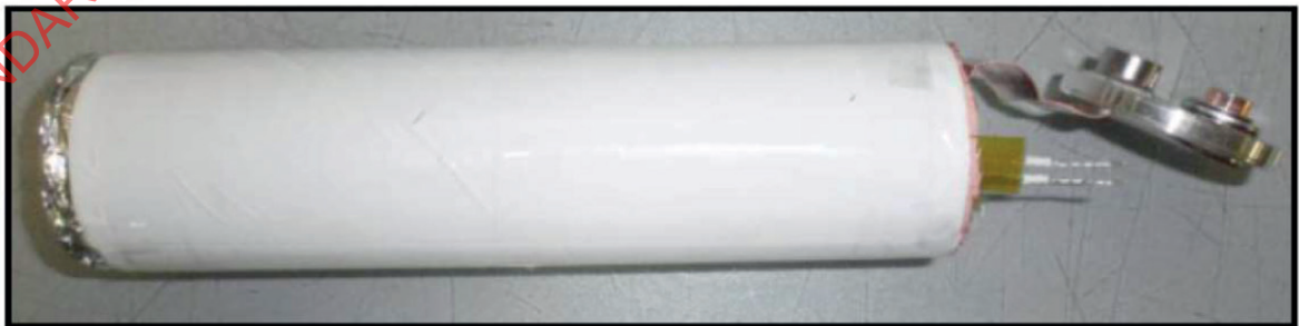
Figure 10 — Example of jelly roll equipped with heater
