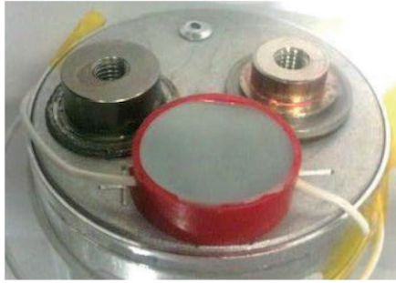
Figure 12 — Example of cell before filling with electrolyte
