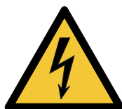
Figure 1 — Marking of voltage class B electric components
