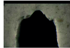
d) Notch insufficiently sharp
