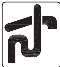
Figure A.2 — Pump-out fitting symbol
