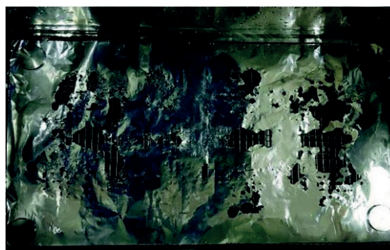
Figure E.3 — Aluminium foil after ultrasonic performance check
